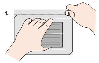
Position the boat package on a solid base. Hold the boats firmly with one hand. With the other hand, grab the plastic tab at the outer edges. The use of gloves is recommended when opening 3M™ Evaporation Boats.
